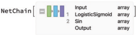
Figure 9-27. NetChain containing two elementwise layers
