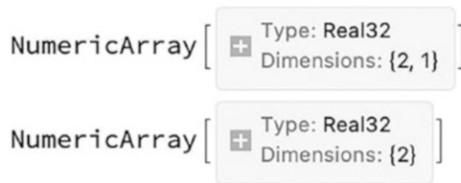
Figure 9-7. Weights and biases of a linear layer
