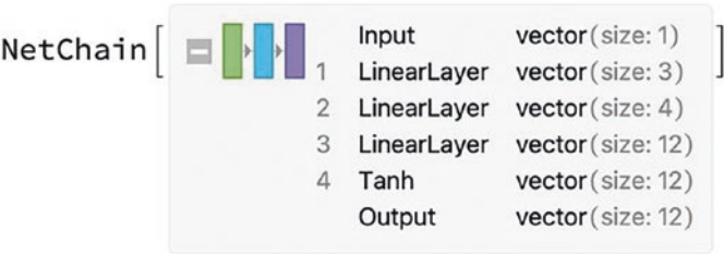
Figure 9-28. NetChain with multiple layers
