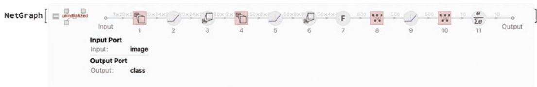
Figure 10-22. NetGraph of the LeNet model
